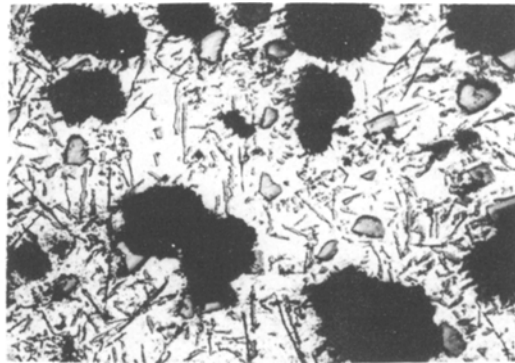
Figure 11 Microstructure of the same casting as Fig. 10 at a height of 0.8 m from the bottom and where alumina particles are present (× 200).
